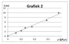
"In grafiek 2 [translated: graph 2] one notices a straight line, therefore a linear relationship between h (m) and  $v^2$  (m<sup>2</sup>/s<sup>2</sup>). Using this graph one can draft an equation (y=ax). First the slope needs to be calculated. Two points on the graph are needed to do so. We use (0,0) and (9.9,0.38). The slope may now be calculated: 0.38/9.9=0.038. In the equation that becomes h=0.038\*v<sup>2</sup>."
